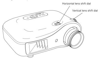
Note: You can display a test pattern to help adjust the image position by pressing the Pattern button on the remote control. Press the Pattern button again to turn off the test pattern.
