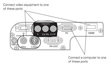
If you connect to the Component port, be sure to select the correct Input Signal setting for your equipment, or the image may not display properly (see page 23).
