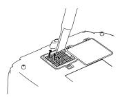
5. If you need to replace the filter, release the tab and lift up the cover.
