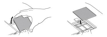
7. To replace the cover, insert the tabs and press down until the cover clicks into place.
