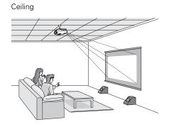
Ideally, place the projector at a height where its lens is between the top and bottom of the screen. That way, you can keep the projector level and use the vertical lens shift dial to position the image. This produces the best-looking picture.
